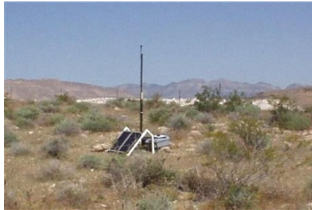
Figure 2-6. Typical Installation of the DustTrak Sampler and Sample System
